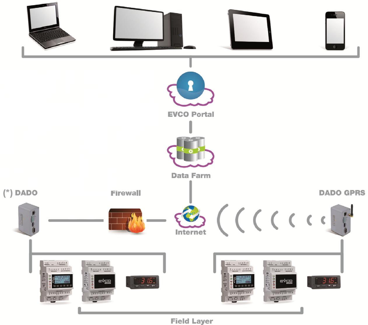
(\*) : An external Wi-Fi adapter can be used for wireless connection to a Wi-Fi Hot Spot.
