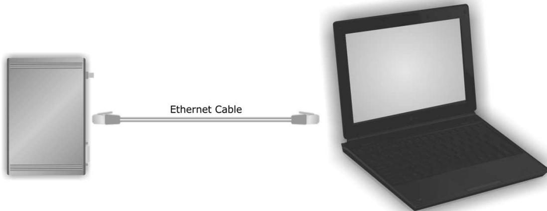
Depending on the PC, a special Ethernet cross cable maybe required. Modern PCs usually don't require this, so in many cases also a common Ethernet cable can be used.
