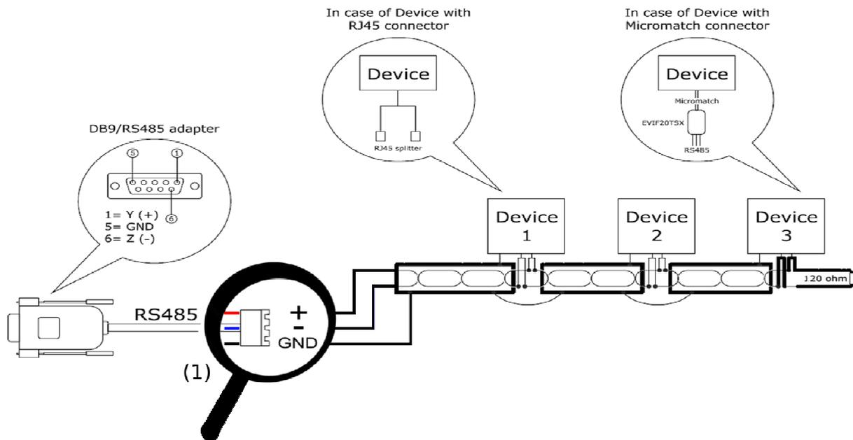
Consult the specification for each device, if it can be connected directly in RS485 or if it need an adapter.
